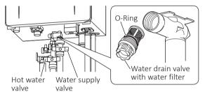
2. With a bucket ready, remove the water drain valve.
